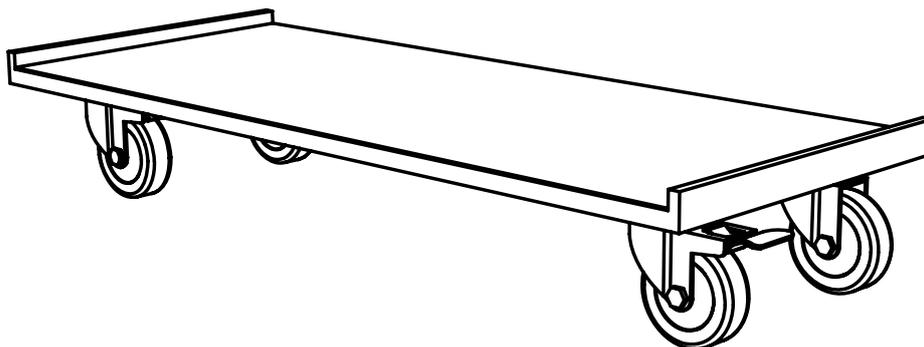
The WLA-12 Dolly should always be used when flying a WLA-12 line array system. Each WLA-12 Dolly will hold a single WLA-12 element. The WLA-12 Dolly helps to protect the WLA-12 element and aid the connection and flying process.
