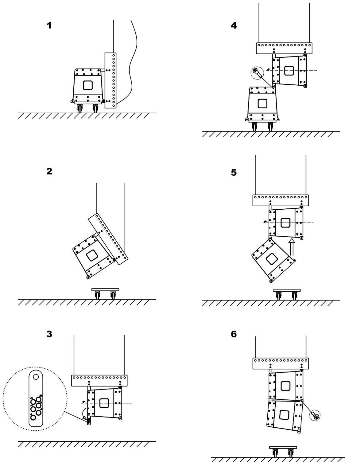
**THE WLA-12 AND FLY FRAME IS CERTIFIED TO HOLD A TOTAL WEIGHT (INCLUDING THIRD PARTY HARDWARE) OF 750KG. 12 ELEMENTS CAN BE FLOWN WITH A SAFETY FACTOR OF 5.7.**
