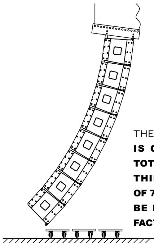
THE WLA-12 AND FLY FRAME IS CERTIFIED TO HOLD A TOTAL WEIGHT (INCLUDING THIRD PARTY HARDWARE) OF 750KG. 12 ELEMENTS CAN BE FLOWN WITH A SAFETY FACTOR OF 5.7.
