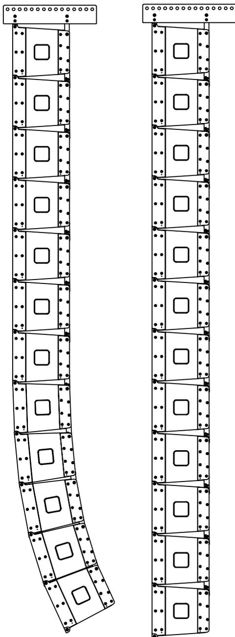
**THE WLA-12 AND FLY FRAME IS CERTIFIED TO HOLD A TOTAL WEIGHT (INCLUDING THIRD PARTY HARDWARE) OF 750KG. 12 ELEMENTS CAN BE FLOWN WITH A SAFETY FACTOR OF 5.7.**
